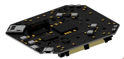
Ocelot is a high-speed, ultra customizable, Systemon-Module (SoM) based upon the Xilinx Zynq®-7000 All Programmable System-on-Chip (SoC). Designed with multi-processor footprint compatibility, the Ocelot offers Single-core ARM® Cortex®-A9 performance with the XC7Z007S or XC7Z014S Zynq®-7000 All Programmable SoC, or Dual-core ARM® Cortex®-A9 performance with the XC7Z010 or XC7Z020 Zynq®-7000 All Programmable SoC.
